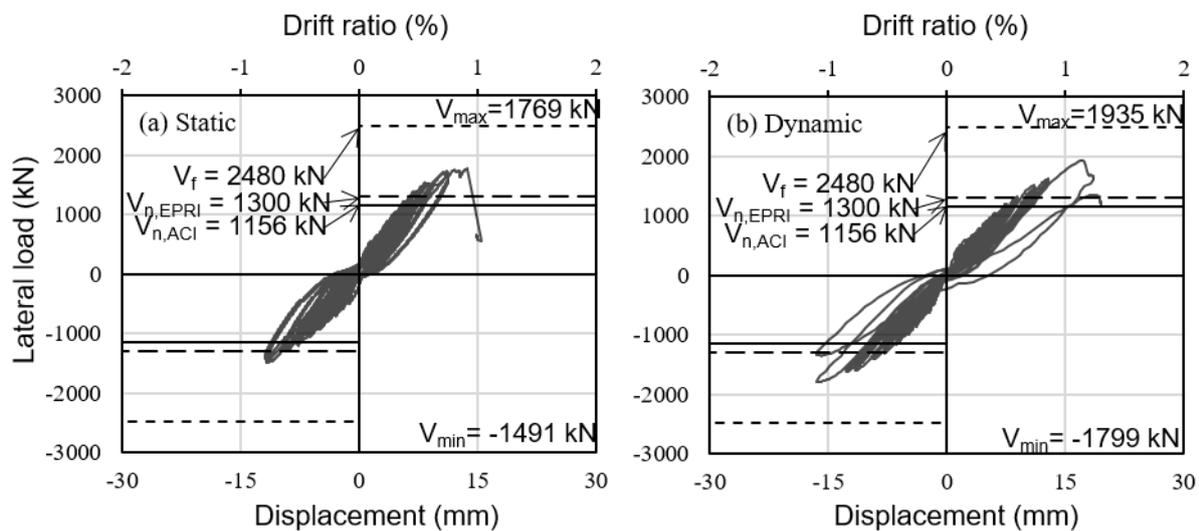
**Fig 2.** Load-displacement relationship
